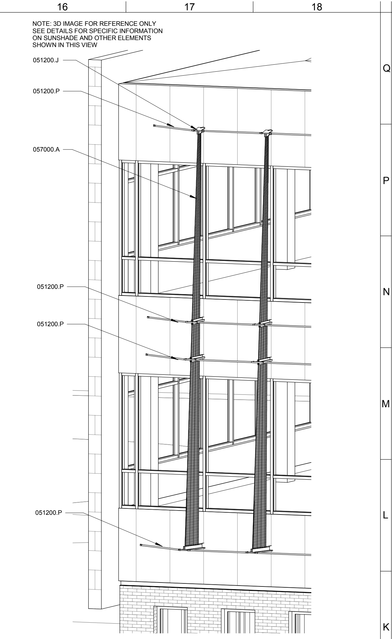
K16 SUNSHADE - WEST VIEW SCALE: NO SCALE OTHER SIDES SIMILAR
