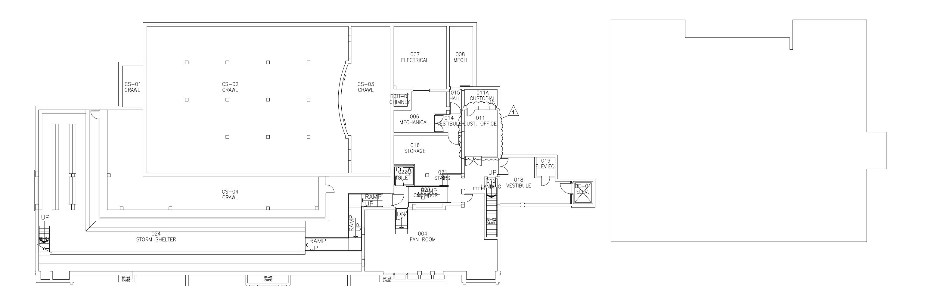
HATCHED AREAS TO HAVE EXISTING FLOORING REMOVED. PERFORM MINOR FLOOR PREP, AND INSTALL NEW CARPET.
